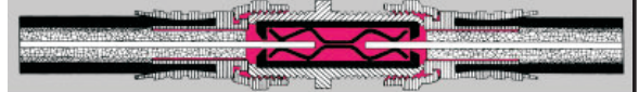
Cross Section of f-splice: RED indicates internal air voids filled with STUF
